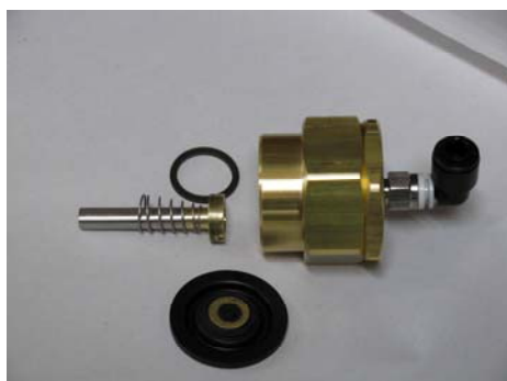
Half Flush Diaphragm Actuator
