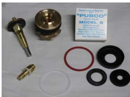
The valve body and main casting components are made from certified gunmetal or red brass (85 to 88% copper). This provides the best possible life for the body, seats and inner valve components as the nominal zinc content is 5%. In stable waters this should give a service life of 20 to 30 years.
